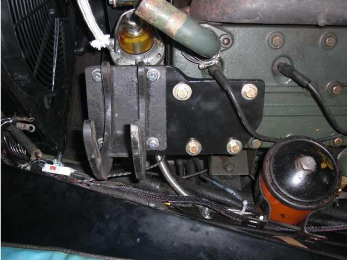
Notice the plate required a cut-out to clear the #1 sparkplug opening, and another to clear the 3rd lower head bolt.
