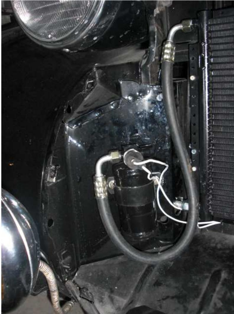
For cooling, I removed the complete engine-driven cooling fan and its mount, and replaced it with an electrical 16" "puller" fan, mounted on the engine side of the radiator. This frees up the fan pulley groove on the crank pulley, which can then serve as the dedicated pulley drive for the compressor.
