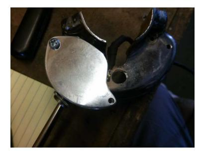
Then the entire piece went to the polishing wheel for a mirror finish, and was finally attached to the back of the turn signal housing with a couple of machine screws:
