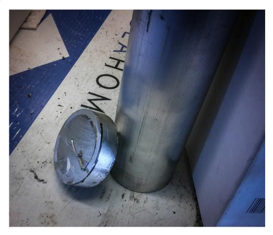
This hunk of aluminum then went to the milling machine, where a recess in the back side was milled, and the piece itself was cut to a suitable shape to mate with the turn signal housing:
